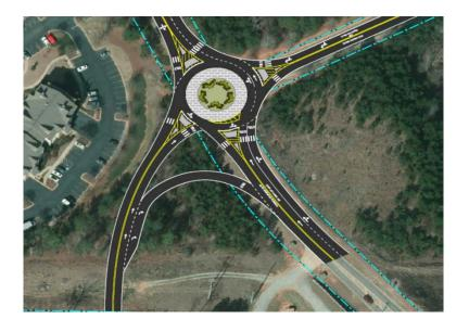
This project consists of constructing a roundabout at Stillwood Drive, eliminating the 3 way stop and creating access for a future development. The Funding will be SPLOST 2019.
