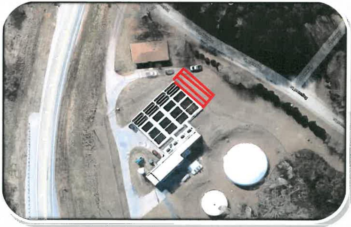
**New 250,000 gallon aerated Digester at the Water pollution Control Plant. The Digester is used to break down solids that enter the plant and helps convert them to the beneficial final product Biosolids. This Digester will be the same as the two added in 2005 and will provide the ability to create stage digestion providing for fewer solids having to be converted to Biosolids and reducing costs over the next several years.**
