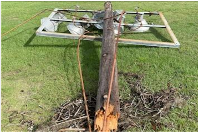
Rotted light poles removed in 2023
